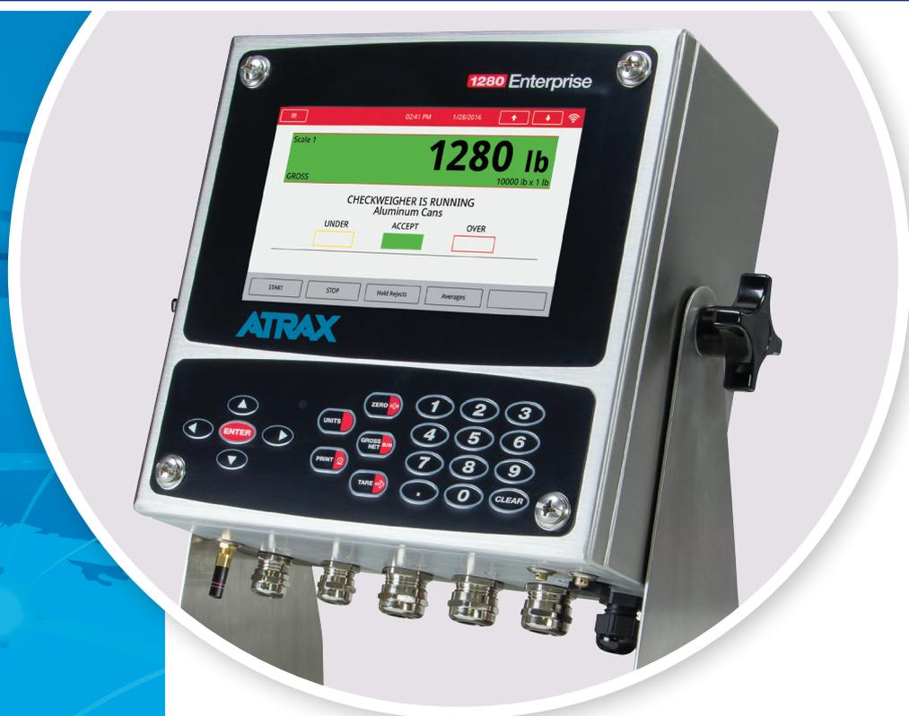
The Atrax Model 1280 Enterprise is an advanced multi-function digital weight indicator, with multiple connectivity options, inputs for up to 8 scales and multi-interval weighing functions. Use this indicator for specialised applications which require special programming or diverse communication options such as Profinet or Wi-fi.
