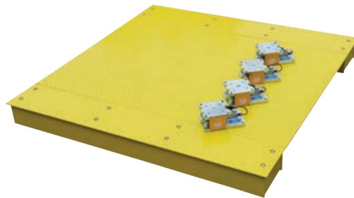
Available with safety non-skid tread plate (chequer plate) or smooth plate top surface. The welded steel frame is completely sand blasted, and painted with a corrosion resistant primer, finished with a durable two pot epoxy paint top coat. A hot dip galvanised finish is also available.
