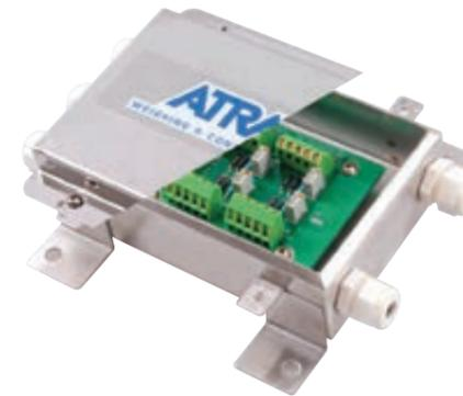
The Atrax LC-650-JB Junction Box provides summation and calibration sensitivity matching for up to six load cells in a weighing system, and combines the weight signals into a single output. Atrax's design minimises interaction between load cell channels and zero points and employs quick connect wire terminals and 25 turn fine adjust trim-pots, all of which means quicker and simpler installation and commissioning of your system.
